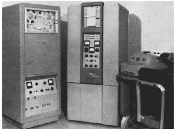
Fig. 4. Computer system (left to right): incremental pulse reader, digital computer, and typewriter.
