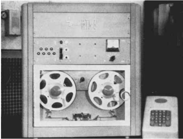
Fig. 3. Incremental pulse recorder (magnetic tape) with keyboard.
